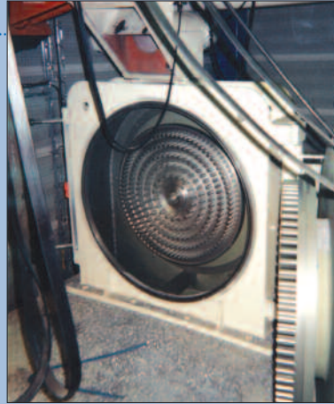
FNG.4 Grinder Pin plate made in Tungsten carbide
