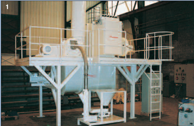
(1) - Grinding plant FL.3 for pure icing sugar with agitated buffer hopper with capacity 1000 l. Crystal sugar feeding by vacuum extraction.
