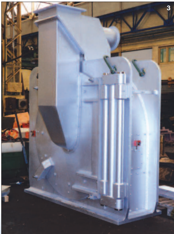
(3) - FNG.7 Grinder – Hammer Plate Ø rotor : 1500 mm Installed power: 315 KW Flow rate: 37 T/h Product: plaster
