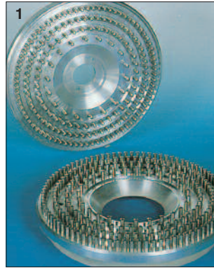
(1) - Grinding equipment Static and rotating plate
