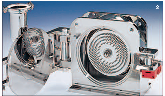
(2) - FPX Mill – Pharma design with easy dismantable pin stator Installed power: 3 KW Flow rate: 50 kg/h - < 100 µm Product: pharmaceutical principles
