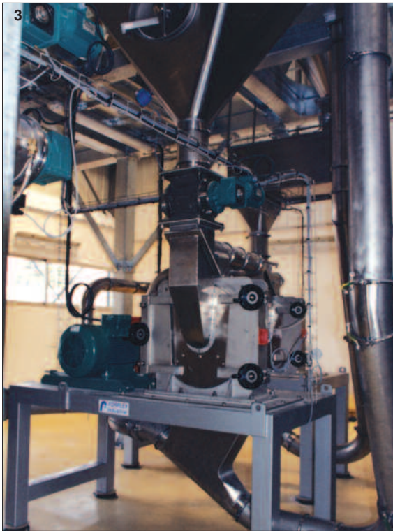
(3) - FNG.3 Grinder on pneumatic transport box Installed power: 37 KW Flow rate: 1T/h Product: casein
