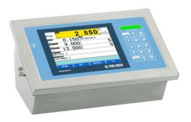
Digital weight indicator with a big touch screen display, suitable for advanced industrial applications. It allows the visualization of all the weighing data and the customization of the screens, simplifying the user operations. Fitted with 3 serial ports, transmission protocols for data communication, completely configurable printouts, integrated alibi memory, and port for connection to barcode/badge reader. CE-M approvable (OIML R-76 / EN 45501).
