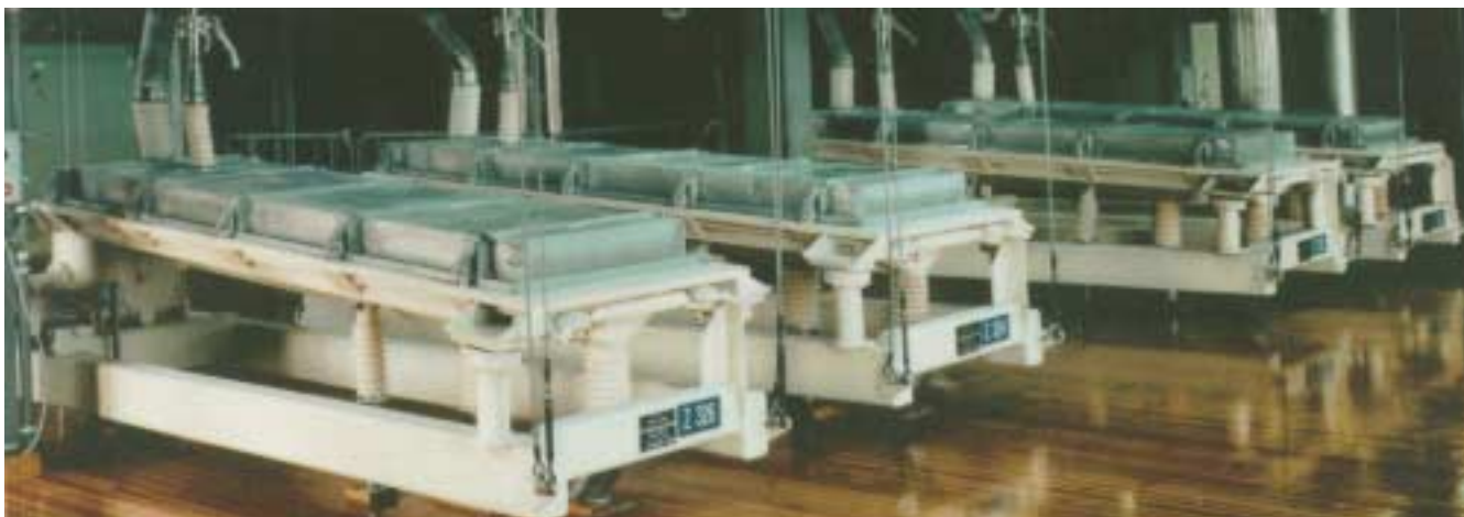
Bank of ten Model 82-SAN ROTEX Screeners for sizing citric acid.
