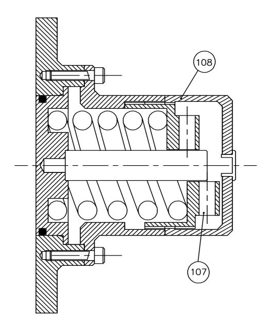
Fig 12 Spring Loaded Integral Pressure Relief Valve with Manual Lift OL1, OL2, OL3 (S1, S2, S3) Typical.
