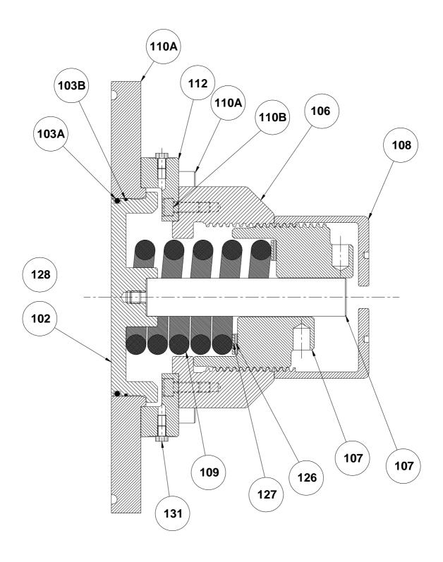
Fig 13 Spring Loaded Integral Pressure Relief Valve with airlift OL1, OL2, OL3 (S1, S2, S3) Typical.
