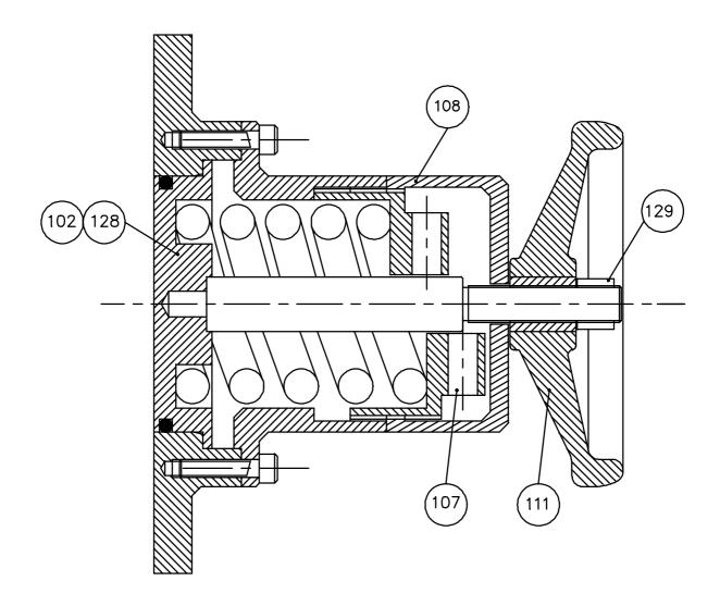
Fig 12.5 Spring Loaded Integral Pressure Relief Valve OL4 (S4) Typical.
