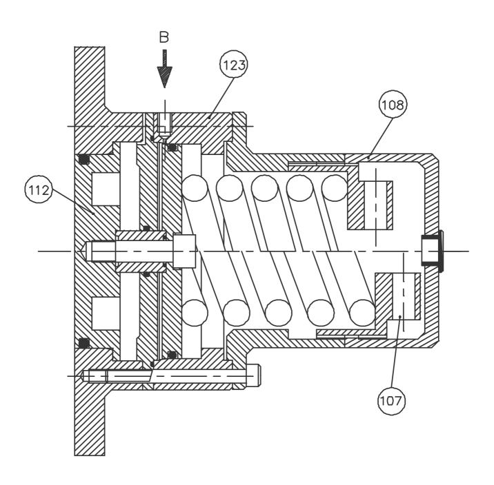
Fig 14 Air Loaded Integral Pressure Relief Valve with airlift OL1, OL2, OL3 (S1, S2, S3) Typical.
