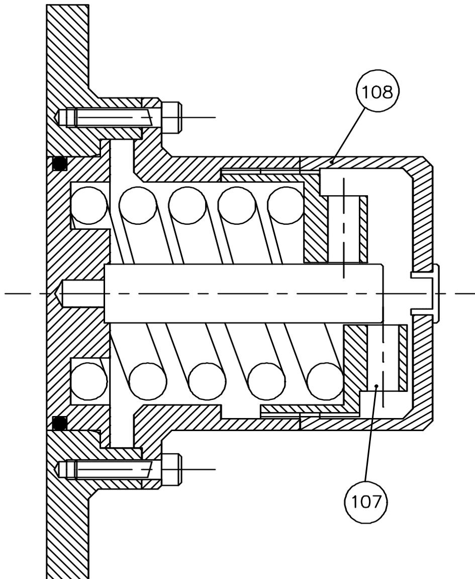
Fig 12 Spring Loaded Integral Pressure Relief Valve with Manual Lift
