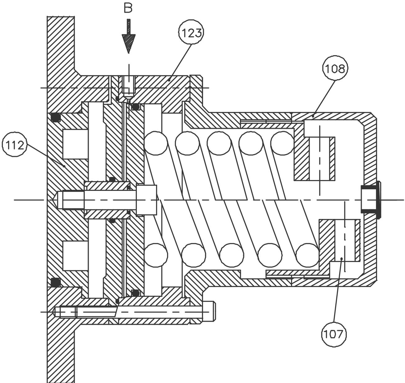
Fig 14 Air Loaded Integral Pressure Relief Valve with airlift OL1, OL2, OL3 (S1, S2, S3) Typical.
