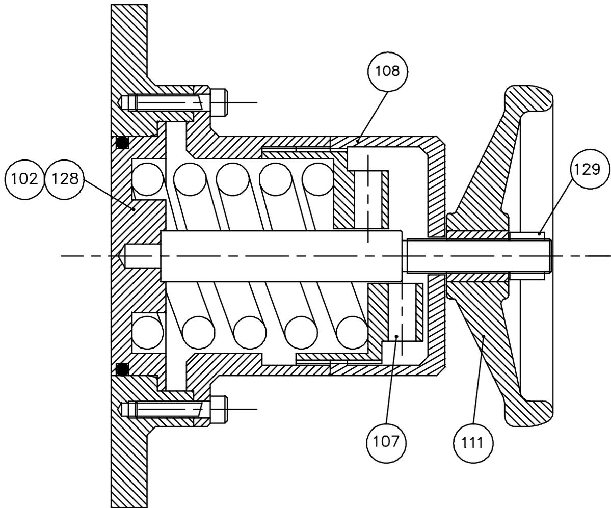
Fig 12.5 Spring Loaded Integral Pressure Relief Valve OL4 (S4) Typical.
