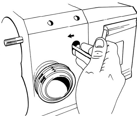
Insert seal extraction tool into the drain/leakage detection slots at the side of the rotorcase and apply a twisting action to remove the seal face (item 46 see fig 29 page 47).
