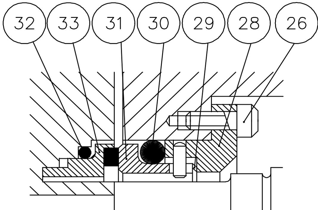
Read the General Procedures to prepare for seal installation refer to section 4.3.1 before assembly Ensure that all seal components are clean and grease free.
