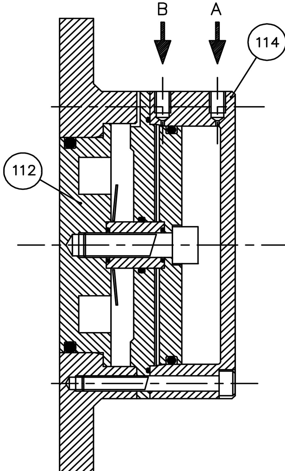
Fig 14.5 Air Loaded Integral Pressure Relief Valve with airlift OL4 (S4) Typical
