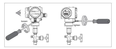
Loosen the screw underneath the connection compartment to rotate the housing.
