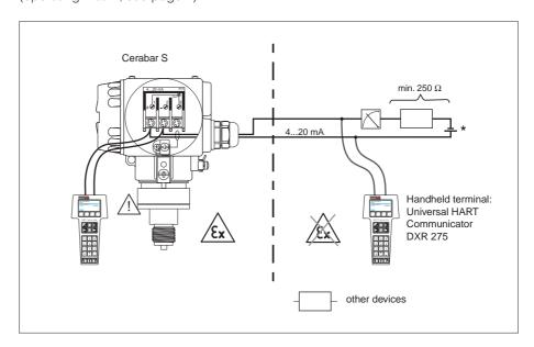
The HART Communicator DXR 275 can be connected anywhere along the 4...20 mA line.
