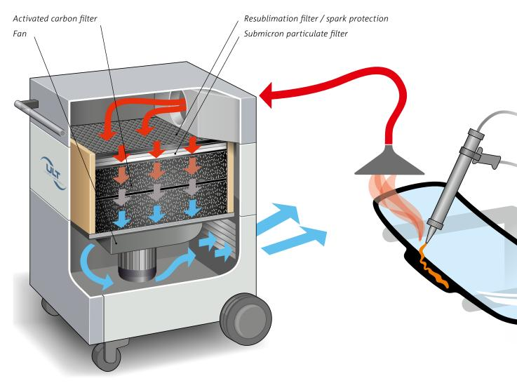
ACD type devices are saturation filter units.
