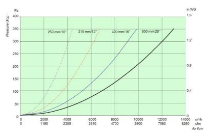
Pressure drop for Inlet and outlet. Actual working pressure will depend on application and dimensioning. Dimensional typical pressure drop for FilterMax 1200 Pa (5" WG)
