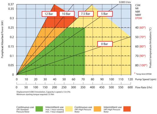
Flows are typical and were measured with water at 20°C with no suction lift or discharge pressure. Actual flows will vary according to suction conditions, discharge pressure and normal component production tolerances.
