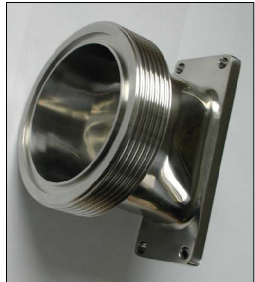
Rectangular to round adaptor finished with screwed connection
