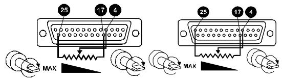
Note: As the remote potentiometer utilises the 0-10V range the speed response is only over  $^{10}/_{12}$  the potentiometer's electrical travel. The signal overload illuminates at this point and there is no further increase in speed.
