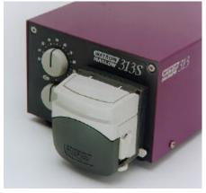
To remove the pumphead push the bayonet plate locking lever back towards the rear of the drive and turn the pumphead anti-clockwise until it is freed from the bayonet plate fittings.
