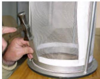
*Assembly and clamping of the collar*
