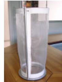
*Fit the nylon on the framework, taking care of the arrow direction indicated on this nylon*
