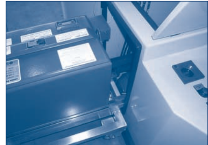
Quick battery exchange with telescoping drawers
