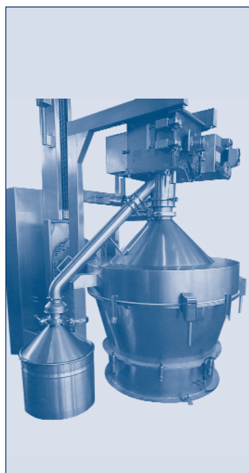
Discharging of a product container with calibration and adding of flow enhancer
