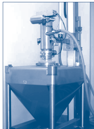
Container filling by vacuum conveyor system
