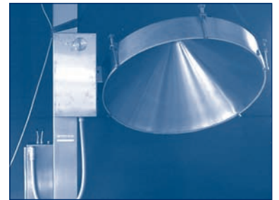
Filling and discharging cone for product containers (vortex layering system)
