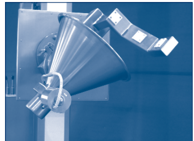
Drum fixing by flange on the funnel with torque support
