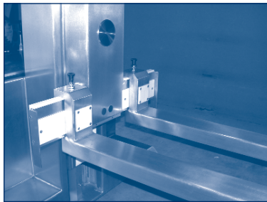
Adjustable carrier fork for various container types
