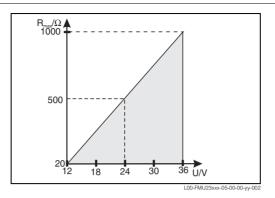
The maximum load  $(R_{max})$  depends on the supply voltage (U).
