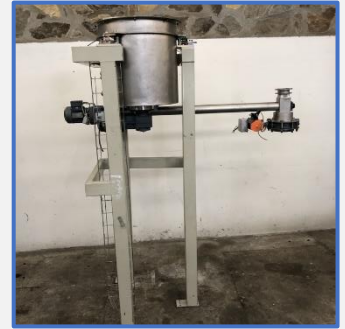
Trémie de dosage 170L inox S/S screw feeder
