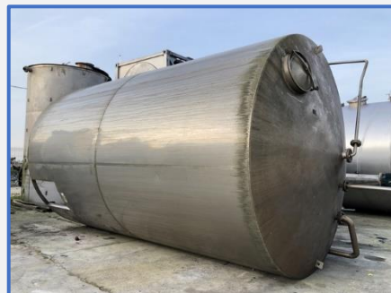
40 000 LITRES inox, calorifugée Verticale / Insulated S/S vertical tank
