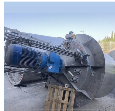
Cuve de fabrication 3000L ABB - 55 KW S/S process tank
