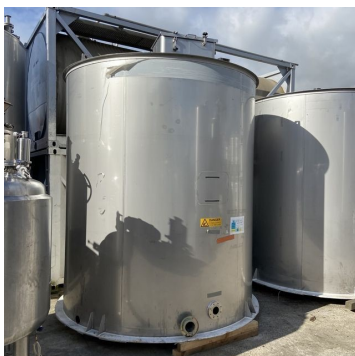
3 cuves inox 17 000 litres S/S tanks
