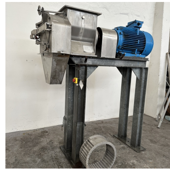
Broyeur râpe 22KW inox S/S grater grinder
