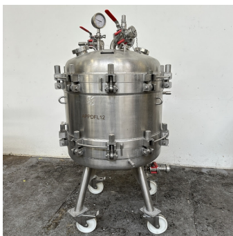
Filtre monoplaque inox Ø 800 mm EUROFILTEC S/S single plate filter
