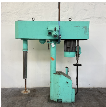
Disperseur RAYNERI 22 KW Lifting head dissolver
