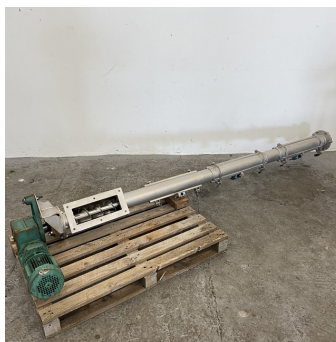
Vis sans fin inox Lg. 2600 mm S/S screw conveyor
