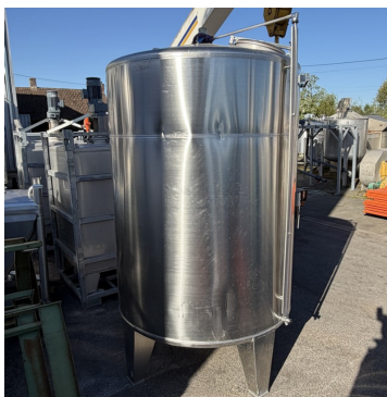
Cuve inox 316L COELHO 4250 litres S/S tank
