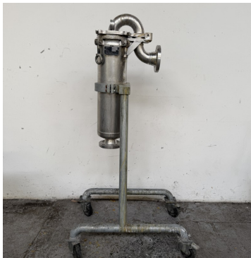
Filtre à poche inox EATON GAF type RB1ASLM Bag filter housing model
