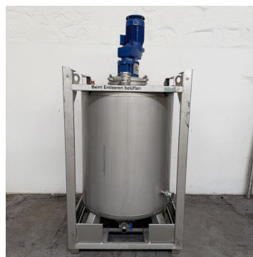
9 containers inox agités 1250 litres UCON S/S agitated tanks
