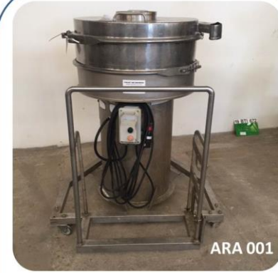
Tamis / Sieving machine SWECO Type LS30D63C
