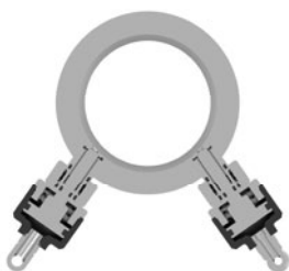
Arrangement of the flushing valves
